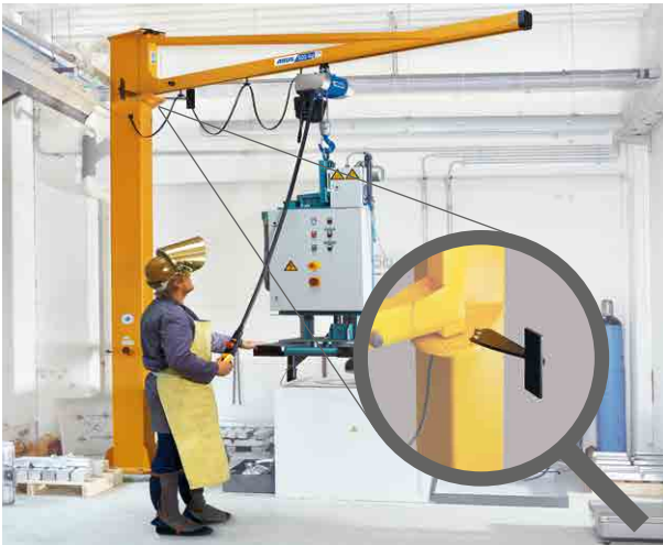
Slewing limit stops, adjustable (Fig. 5)
