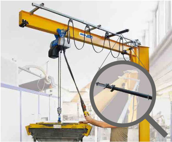
Slewing limit stop - bumper rod (Fig. 4)
