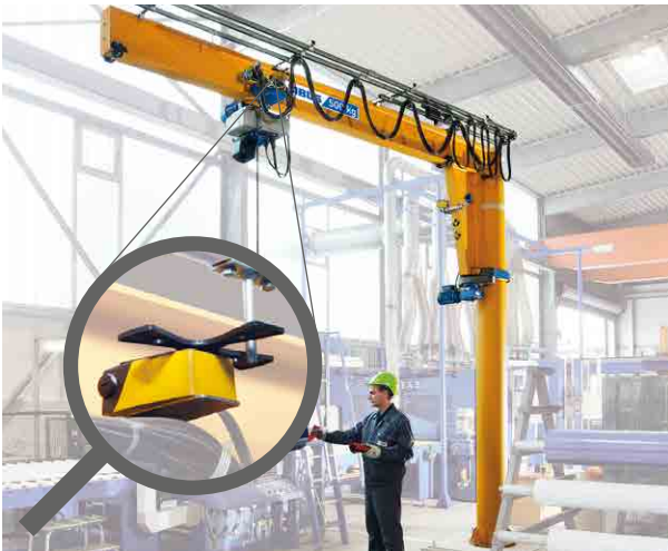
Limit switch for trolley travel (Fig. 8)
