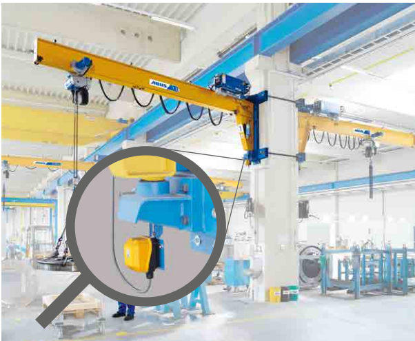
Slewing limit switch, VW (Fig. 7)
