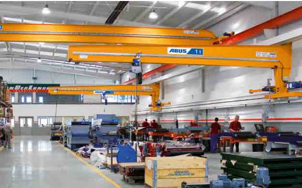
ABUS EWL wall travelling crane
